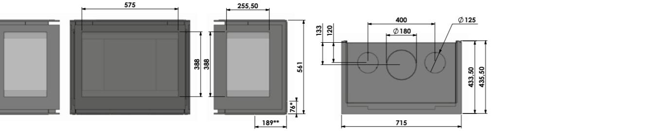
Unilux-6 270 Three sided - inbouw kader / built-in frame / cadre encastrable / Einbaurahmen - Measurements under reservation
