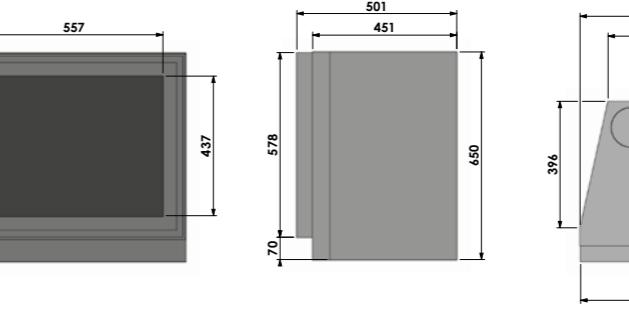
Universal-6 75 - inbouw kader / built-in frame / cadre encastrable / Einbaurahmen
