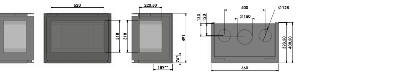
**Unilux-6 265 Three sided - inbouw kader / built-in frame / cadre encastrable / Einbaurahmen**
