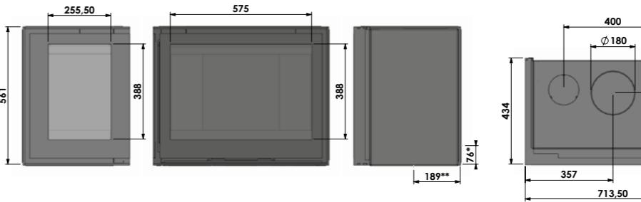
Unilux-6 270 Left - inbouw kader / built-in frame / cadre encastrable / Einbaurahmen - Measurements under reservation
